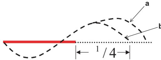
**Figure 5.** COSINE TAPERING OF CORRECTION OFF THE END OF A PATH SECTION. THE CORRECTION FROM THE DECOMPOSED FFT WAVENUMBER (A) IS REDUCED TO ZERO AT A QUARTER-WAVELENGTH DISTANCE FROM THE END OF THE SUTURE PATH SHOWN AS A SOLID HORIZONTAL LINE.
