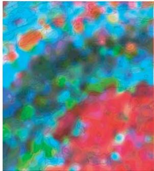
**Figure 4.** TERNARY MAPS PROVIDE A USEFUL MEANS OF DISPLAYING THE INTERRELATIONSHIPS AND SPATIAL RELATIONSHIPS BETWEEN THREE ELEMENTS SIMULTANEOUSLY. THIS FIGURE DEPICTS A THREE-GRID COMPOSITE (TERNARY) OF ZIRCONIUM (CYAN), NICKEL (MAGENTA), AND COBALT (YELLOW) USING A LOGNORMAL CONTINUOUS COLOR DISTRIBUTION. THE OVERLYING DXF DRAWING REPRESENTS THE INFERRED GEOLOGY OF THE AREA.
