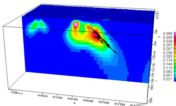
**Figure 7:** An EW section through the recovered MVI model amplitude at the Osborne property with the now known mineralization shown in black. The color bar gives the normalized amplitude in SI. The axes are in metres.
