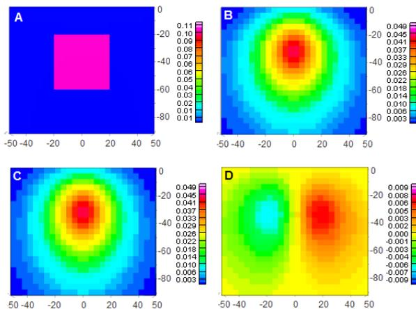
**Figure 4:** (a) A cross section through the true model, (b) the recovered amplitude of the magnetization vector, (c) the amplitude of the perpendicular-to-earth-field components of the magnetization, (d) the projection of the magnetization on to the earth field direction. The colour scales indicate the MVI magnetization in normalized to SI (see text).
