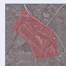
Figure 6: Orthophoto with prospective area showing proposed sampling region with survey grid created with Geosoft survey plan wizard.
