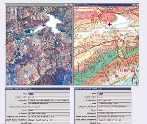
Figure 4: Landsat imagery accessed in Geosoft via ER Mapper plug-in and corresponding geology map. The cross-hair symbol represents a dynamic link between datasets in different projections. Projection information is shown below.
