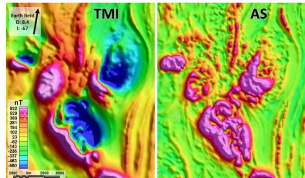
Figure 1. TMI and analytic signal (AS) of the area including the Black Hill Norite.
