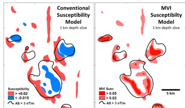
Figure 2. Comparison of conventional susceptibility with MVI susceptibility model at a plan depth slice of 1 km. An outline of the anomalously high analytic is shown as a black line for spatial reference.
