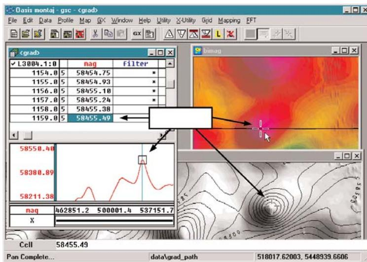
**Figure 8:** A DATA LINK ALLOWS AN INTERPRETER TO SELECT AN ANOMALY ON AN IMAGE AND IMMEDIATELY SEE THE ORIGINAL DATA IN THE SPREADSHEET VIEW AND ON OTHER MAPS
