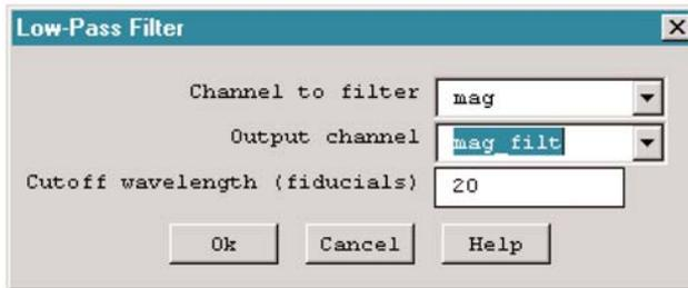
**Figure 6:** SAMPLE CONTROL DIALOGUE PRESENTED BY A LOW-PASS FILTER GX. ALL PROCESSING FUNCTIONALITY IN OASIS IS CARRIED OUT BY GXs, WHICH CAN BE DEVELOPED BY END-USERS.
