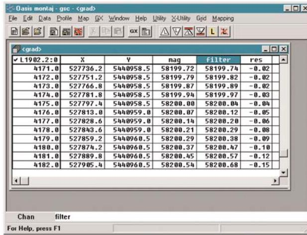
**Figure 3:** AN OASIS MONTAJ PROJECT WORKSPACE SHOWING AN OPEN DATABASE DISPLAYED IN A SPREADSHEET. THE SURVEY LINE NUMBER (TYPE NUMBER.VERSION:FLIGHT) IS SHOWN IN THE TOP LEFT CORNER AND THE LINE FIDUCIAL IS IN COLUMN BELOW THE LINE NUMBER. CHANNELS ARE AUTOMATICALLY RESAMPLED IN ORDER TO BE DISPLAYED WITH OTHER CHANNELS.
