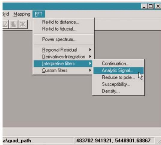
**Figure 7:** THIS SHOWS THE MENU ASSOCIATED WITH THE 1-D FFT GX SUITE. EACH MENU ITEM IS CONNECTED TO A SEPARATE GX PROCESS.
