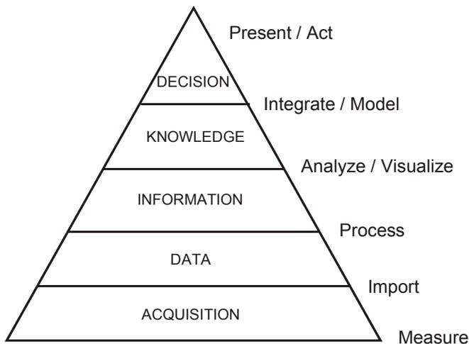
At the base of the pyramid is a measurement or sample. The acquisition component considers all relevant constituents related to data gathering, such as survey design, operator effectiveness, and physical or electronic collection of measurements or samples.
