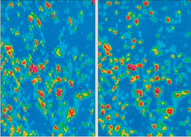
Another type of positioning error that can be controlled in the field is related to the EM61 system. With this instrument, losses in air pressure in the tires can reduce the circumference of the wheels on which the instrumentation is mounted. The effect is a mispositioning of the measuring point. Standardized field practices can reduce this type of effect. The manufacturer (Geonics) now supplies the wheels with solid rubber tires to avoid this problem.
