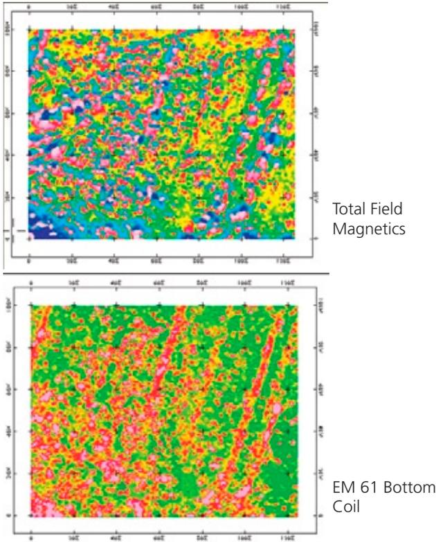
directional gridding products are shown in Figure 4. Either method can yield good results although the bidirectional method may stretch extreme values located on single lines perpendicular to the line direction. This results in a distorted anomaly shape. Alternately, the minimum curvature method is optimized for random data and does not honor line-to-line correlation particularly well.
