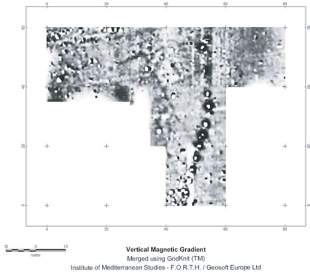
**Figure 2.** VERTICAL MAGNETIC GRADIENT GRIDS MERGED USING THE GRIDKNIT™ SUTURING TECHNIQUE.
