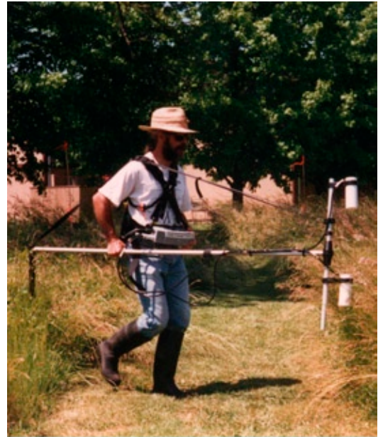
A geometrics g-858 Magnetometer in operation
