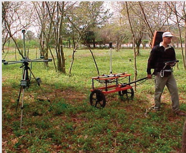
Simple things like instrument noise, steel toed boots, jangling keys in the operator's pocket and flopping cables can all result in inconsistent data, and contribute to faulty decision-making.
