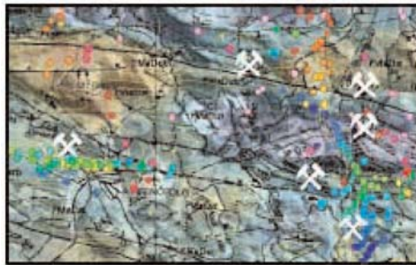
THIS GEOSOFT PRESENTATION COMBINES MAGNETIC DATA FROM A 2 KM WIDE SERVIÇO GEOLÓGICO DO BRASIL (CPRM) DATASET WITH ER MAPPER LANDSAT IMAGERY AND COLOUR-SHADED THORIUM VALUES. GEOLOGY HAS ALSO BEEN ADDED USING THE ER MAPPER PLUG-IN FROM WITHIN OASIS MONTAJ.
