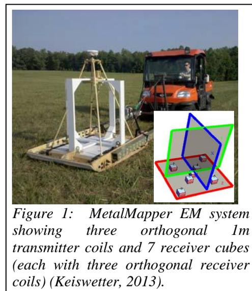
*Figure 1: MetalMapper EM system showing three orthogonal 1m transmitter coils and 7 receiver cubes (each with three orthogonal receiver coils) (Keiswetter, 2013).*
