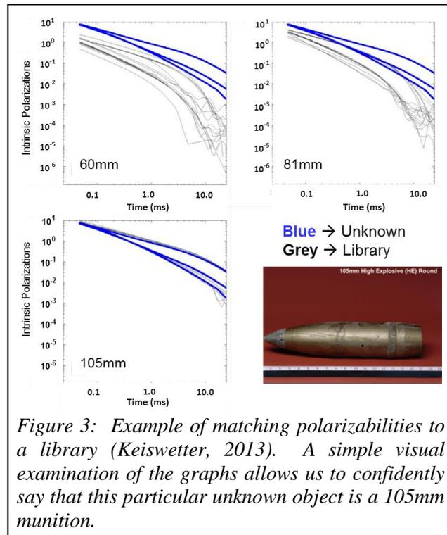
Figure 3: Example of matching polarizabilities to a library (Keiswetter, 2013). A simple visual examination of the graphs allows us to confidently say that this particular unknown object is a 105mm munition.
