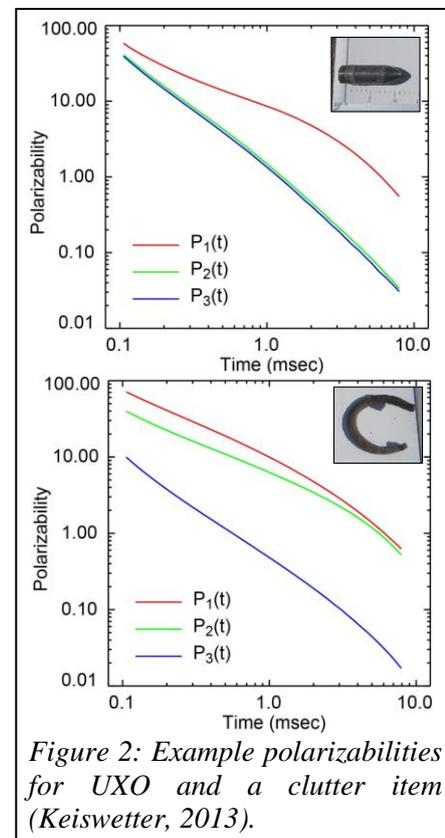
Figure 2: Example polarizabilities for UXO and a clutter item (Keiswetter, 2013).
