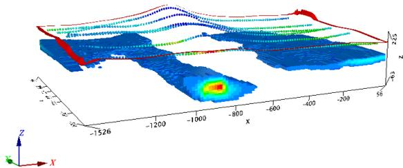
Figure 6. The voxel model recovered by Quasi3D inversion, showing the Maimón orebody (red) and the conductive weathered cover (blue). The voxel threshold is 0.012 S/m.
