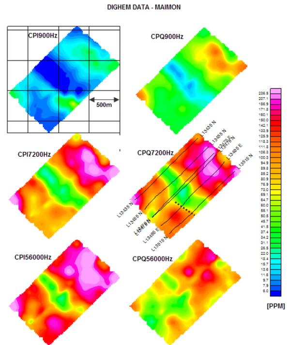
Figure 5. The Dighem data acquired over the Maimón deposit, courtesy of CGG and GlobeStar, shown for the 3 frequencies (900Hz, 7200Hz, 56000Hz), in-phase and quadrature components. The flight lines are superimposed on the CPQ7200Hz response with the surface expression of the deposit (dashed).
