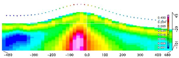
Figure 3. The result of Quasi3D inversion of the LokiAir data simulated over the Sulphide conductivity model used to compare the inversions associated with the layered earth approximation, the full 3D response, and the Quasi3D approximation.
