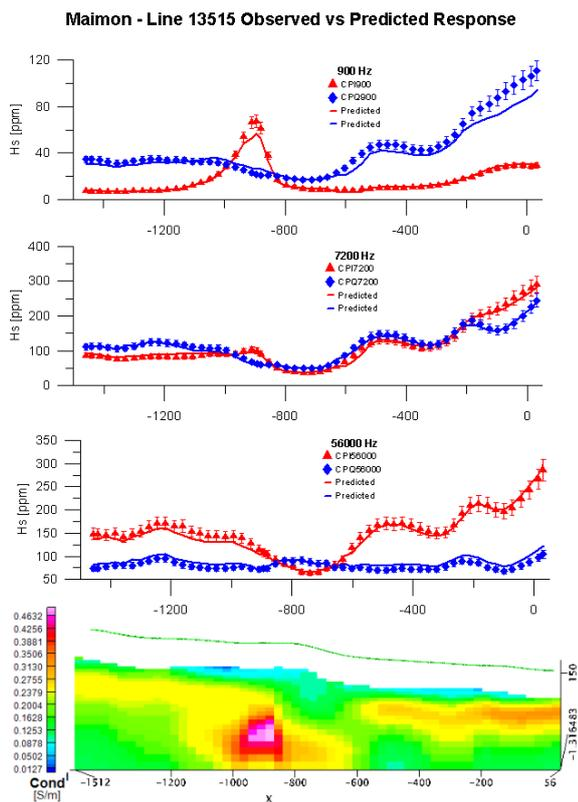
Figure 7. The observed data (symbols) and predicted data (solid) for Line 13515 are shown in the 3 upper panels for the 900 Hz, 7200 Hz, and the 56 KHz Dighem data at Cerro de Maimón. The bottom panel shows the corresponding slice through Quasi3D inversion model.
