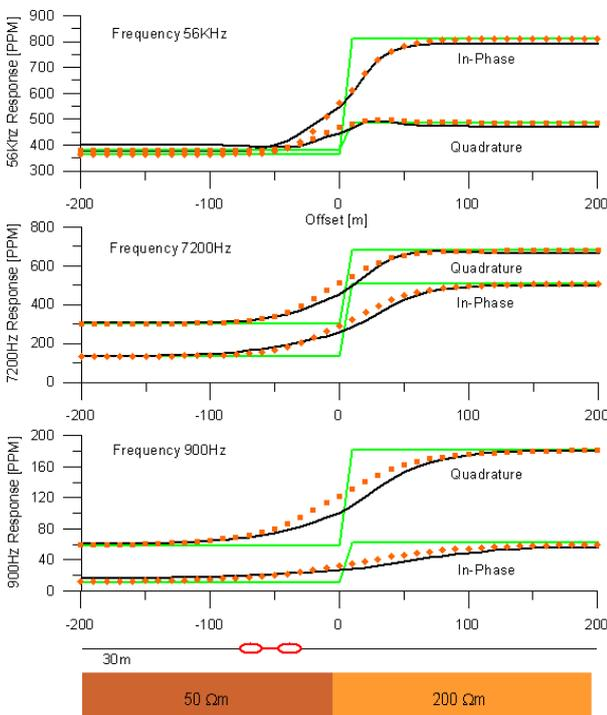
Figure 1. The Quarter space conductivity model used to compare the responses associated the layered earth approximation (green), the full 3D calculation (black), and the Quasi3D response (orange: diamonds for in-phase, squares for quadrature).
