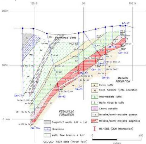
Figure 4. Cross section of the Cerro de Maimón Deposit. Sulphides are massive (red) to semi-massive (hatched). Grid lines are 100m. (Roos et al. 2008)
