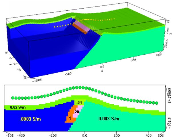
Figure 2. The "Sulphide" conductivity model used to test the Quasi3D approximation. The upper panel shows a 3D perspective, the lower panel shows a section through the centre of the model. The model consists of massive sulphide (magenta), an alteration halo(brown), a paleochannel (lime), a fault, and saprolite cover (green) under an undulating topography.
