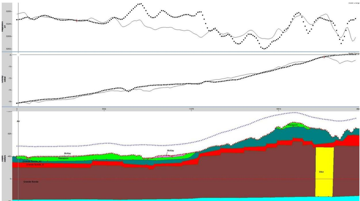
Figure 3. Profile 2 2-D potential field model displaying magnetic and gravity data and geologic interpretations.
