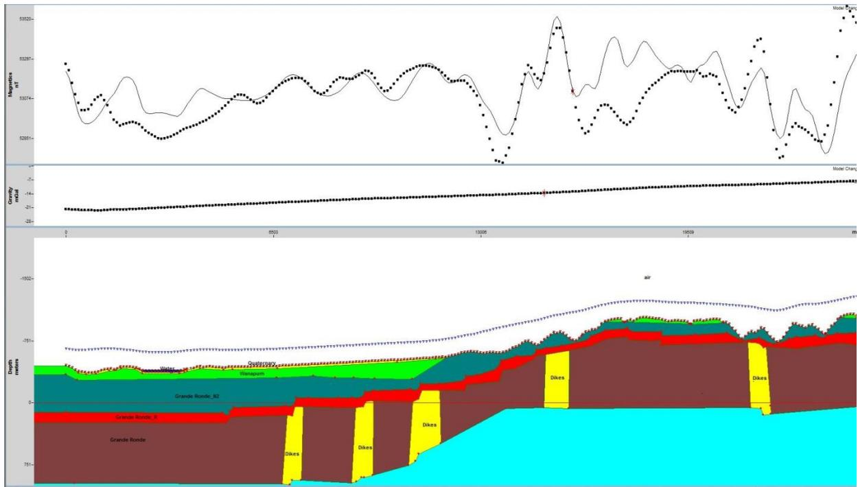
Figure 2. Profile 1 2-D potential field model displaying magnetics and gravity data and geologic interpretations.
